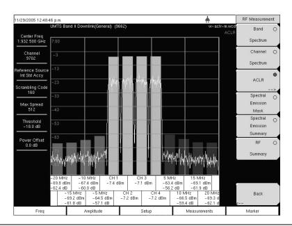
Figure 4-11. ACLR Multi-channel Measurement Example
