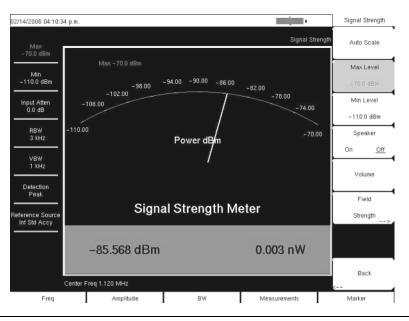
Figure 6-11. Interference Analyzer Mode Signal Strength Display
