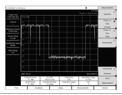
Figure 5-8. EDGE Power versus Time (Frame) Measurement Example
