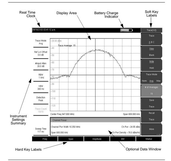
Figure 2-3. Spectrum Analyzer Display Overview
