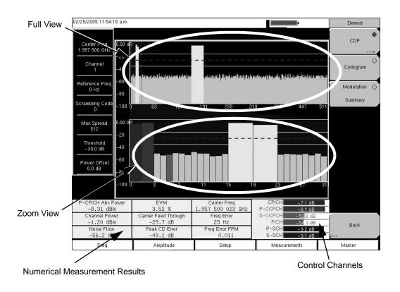
Figure 2-4. WCDMA Signal Analyzer CDP Display Overview
