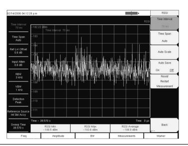
Figure 6-12. Interference Analyzer Mode RSSI Display
