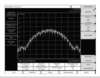
Figure 5-5. GSM Single Channel Measurement Example
