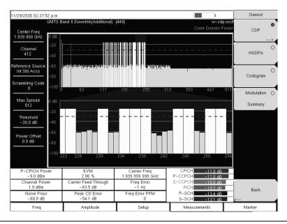
Figure 4-15. WCDMA Code Domain Power Measurement Screen Example
