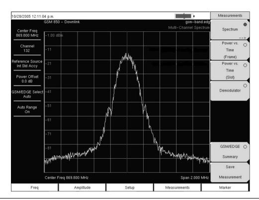
Figure 2-6. GSM Signal Analyzer RF Spectrum Display
