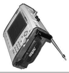
Figure 1-5. Tilt Bail Installed
