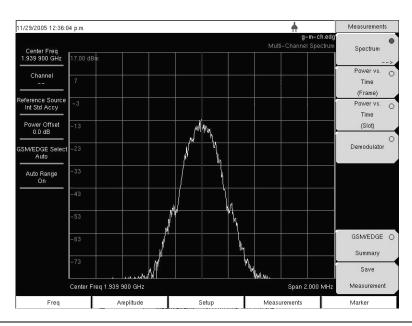
Figure 5-6. GSM Multi-channel Measurement Example
