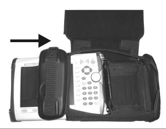
**Figure 1-3. Inserting the Instrument into the Soft Case**
