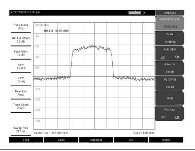
Figure 3-14. Preamplifier Off
