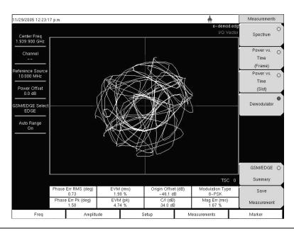
Figure 5-12. EDGE Demodulator Measurement Example
