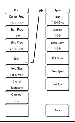
Figure 6-1. Interference Analyzer Mode Freq Menu
