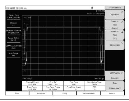
Figure 5-9. GSM Power versus Time (Slot) Measurement Example
