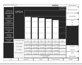
Figure 4-20. OTA Measurement Screen Example
