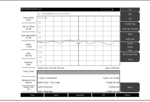
Figure 3-21. C/I Measurement, Results
