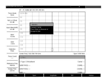
Figure 3-19. C/I Measurement, Ready to Measure the Carrier
