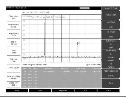
Figure 3-17. Simulated Out-of-Band Spurious Emission Measurement
