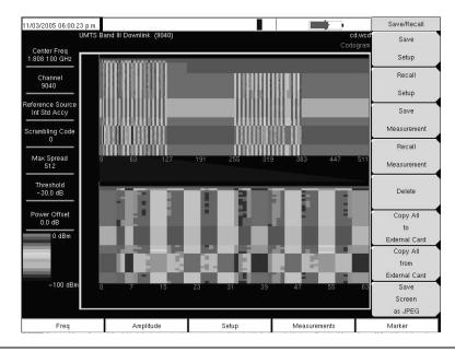
Figure 4-19. Codogram Measurement Screen Example
