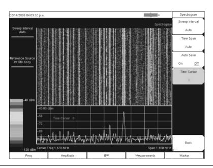
Figure 6-10. Interference Analyzer Mode Sample Spectrogram Display
