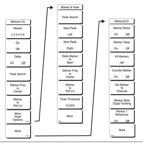
Figure 3-6. Spectrum Analyzer Mode Marker Menu
