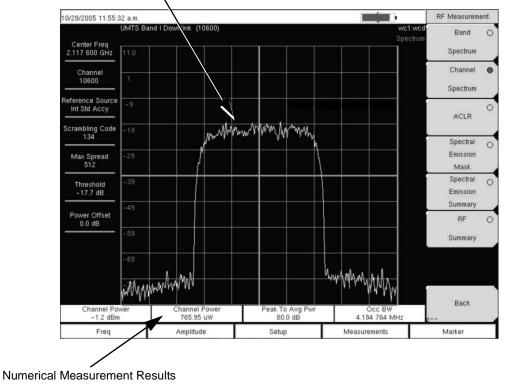
Figure 2-5. WCDMA Signal Analyzer RF Spectrum Display Overview
