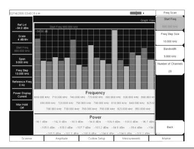
Figure 7-5. Channel Scanner Mode Sample Graph Display
