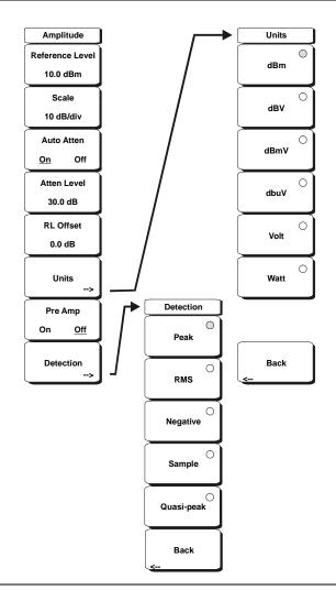
Figure 3-1. Spectrum Analyzer Mode Amplitude Menu
