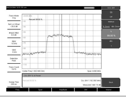
Figure 3-16. Occupied Bandwidth Results Using the % of Power Method
