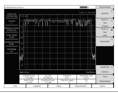
Figure 5-10. EDGE Power versus Time (Slot) Measurement Example
