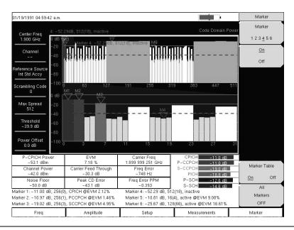
Figure 4-18. Code Domain Power Measurement Screen Example with Markers Activated
