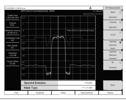
Figure 4-12. Spectral Emission Mask Measurement Example
