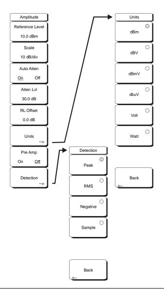
Figure 6-2. Interference Analyzer Mode Amplitude Menu
